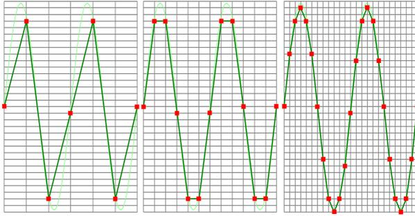
Figure 3.3: The effect of the sampling rate
