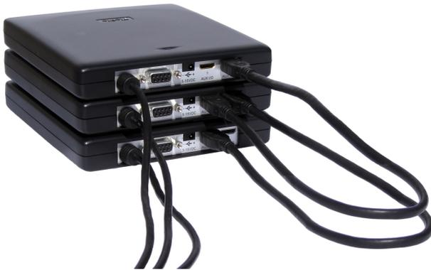
Figure 6.3: Multiple Handyscope HS5s combined
