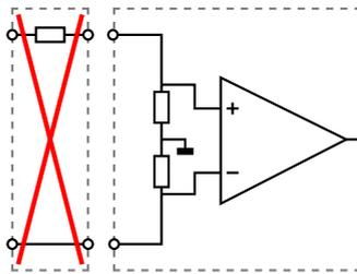
Figure 3.5: Standard probe is mismatch with differential input
