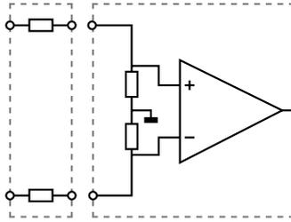
Figure 3.4: Differential attenuator matches with differential input
